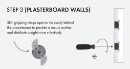
Insert a grip it fixing into each hole and tap with a hammer so its flush with your wall. Use a flat head screwdriver to turn the cam and open the wings for super grip strength.
