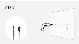
Drill the wall deep enough to accept the wall plugs or GripIt fixings using an **8mm drill bit** for solid walls or a **20mm spade bit** for plasterboard walls.
