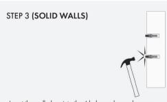
Insert the wall plugs into the 4 holes and use a hammer to tap the wall plugs flush with your wall.
