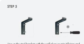
Line up the steel brackets with the wall plugs or grip it fixings and use a screw driver or a drill to screw in the appropriate fixings into position.
