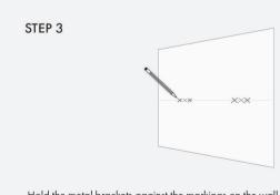
Hold the metal brackets against the markings on the wall and mark where the Gripit fixings need to go, making sure these are level all the way along.
