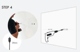
Using a 20mm spade bit, drill a hole on each of the outer marking to accommodate the Gripit fixings.
