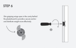
Use a flat head screwdriver to turn the cam and open the wings for super grip strength on every fixing.
