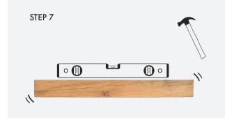
Place a spirit level on the mantel top to check it's level. Minor adjustments can be made by tapping the screws with a hammer.
