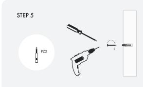
Use a PZ2 drill bit and drill or screwdriver to drive each screw into the wall plugs leaving them protruding approximately  $^1\!\!/\!_4$  of an inch.
