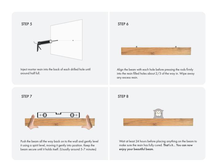
This fixing method can also be used for floating shelves where additional strength is necessary. We recommend the following resin from ScrewFix - FISCHER FIS V HYBRID MORTAR RESIN
