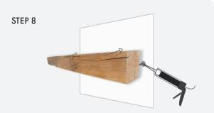
For additional precaution a small amount of silicone or grab adhesive can be applied in the fixing holes to prevent the beam/shelf from becoming loose. Slide the beam/ shelf flush to your wall. As the holes are only 1mm wider than the brackets you'll find it's a tight fit.
