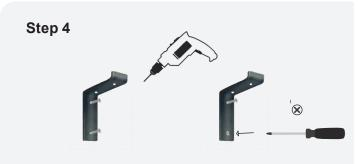
Line up the steel brackets with the wall plugs or grip it fixings and use a screwdriver or a drill with the PZ2 drill bit to screw in the appropriate fixings into position.
