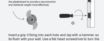
cam and open the wings for super grip strength.
