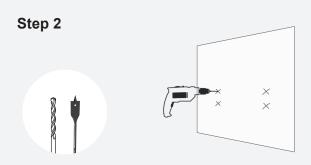
Drill the wall deep enough to accept the wall plugs or grip it fixings using an **8mm drill bit** for solid walls or a **20mm spade bit for plasterboard walls.**
