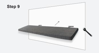
Slide the shelf  $\frac{3}{4}$  of the way onto the brackets so that you can still fit a spanner behind to make any adjustments.
