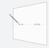
Hold the metal brackets against the markings on the wall and mark where the Gripitfixings need to go, making sure these are level all the way a long.
